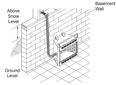
Figure 16 - Basement Installation
